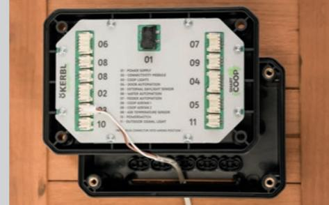
If the connection cable built into the module is not long enough, it can be lengthened using extension cables (items 70629, 70630). Ensure that the connection location is protected from water and dust. The module cable must have only a single extension.
